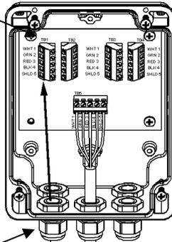
J-Box Illustrated for 4 Load Cell Installation
